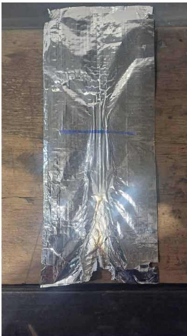
Figure 1: SANS 11925-2 Ignitability test sample after a completed test, flame spread not having exceeded 150 mm. No Flame spread exceeding 150 mm within 20 seconds, filter paper ignited from burning droplets.
